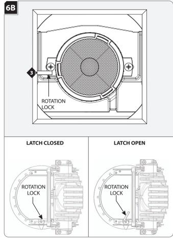
**NOTE:** Lamp housing can rotate 361° horizontally.
