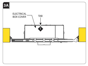
Push the tab on the housing electrical box up and remove the electrical box cover.
